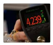
The PCX gauges have user definable upper and lower limits with audible and visual pass/fail warnings allowing the user to compare readings to predefined values. The PCX8-DL can store up to 40 pre-programmed limits whichcan be set for individual readings or for each batch.
