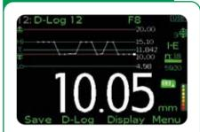
A line trend graph of the last 20 measurements which is updated after each reading.
