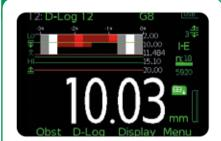
A cross-sectional view of the material being tested is displayed along with readings taken, saved readings, highest (Hi), lowest (Lo) and average (x̄) reading and upper/lower limit values (if set).
