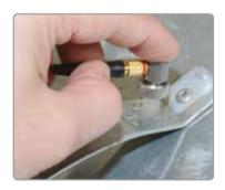
The PCX gauges have a number of calibration options including the 1-Point & 2-Point method and Velocity. Alternatively, the user can select one of 39 pre-set materials stored within the gauge including; aluminium, steel, stainless steel, cast iron, plexiglass, PVC, polystyrene and polyurethane.
