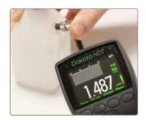
**Interface Echo (IE);** The total thickness from the top of any coating through to the material density boundary (typically the back-wall) is measured. Suitable for measurement of materials between 1.65mm and 25.4mm (0.065" to 1") thick.
