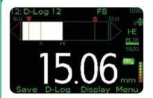
An analogue representation of the current measurement value together with the highest (Hi), lowest (Lo) and average  $(\bar{x})$  reading.
